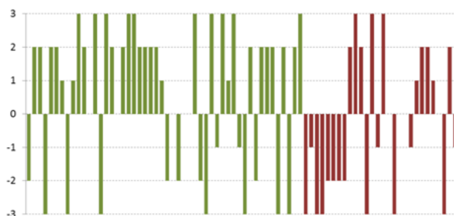
Figure 5.12: The results of the survey of noise comfort (retrofitted buildings – green, non-retrofitted buildings – red); scale from +3 “without annoying street noise” to -3 “street noise is very annoying”
