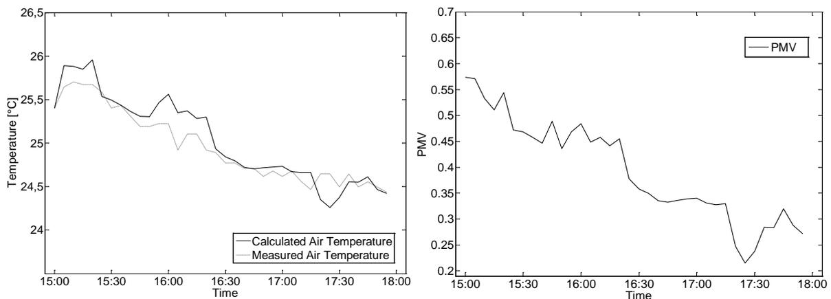
Figure 9: Air temperature comparison (left) and *PMV* of central position inside the room (right) relative to November 4<sup>th</sup> 2010 evening acquisition.
