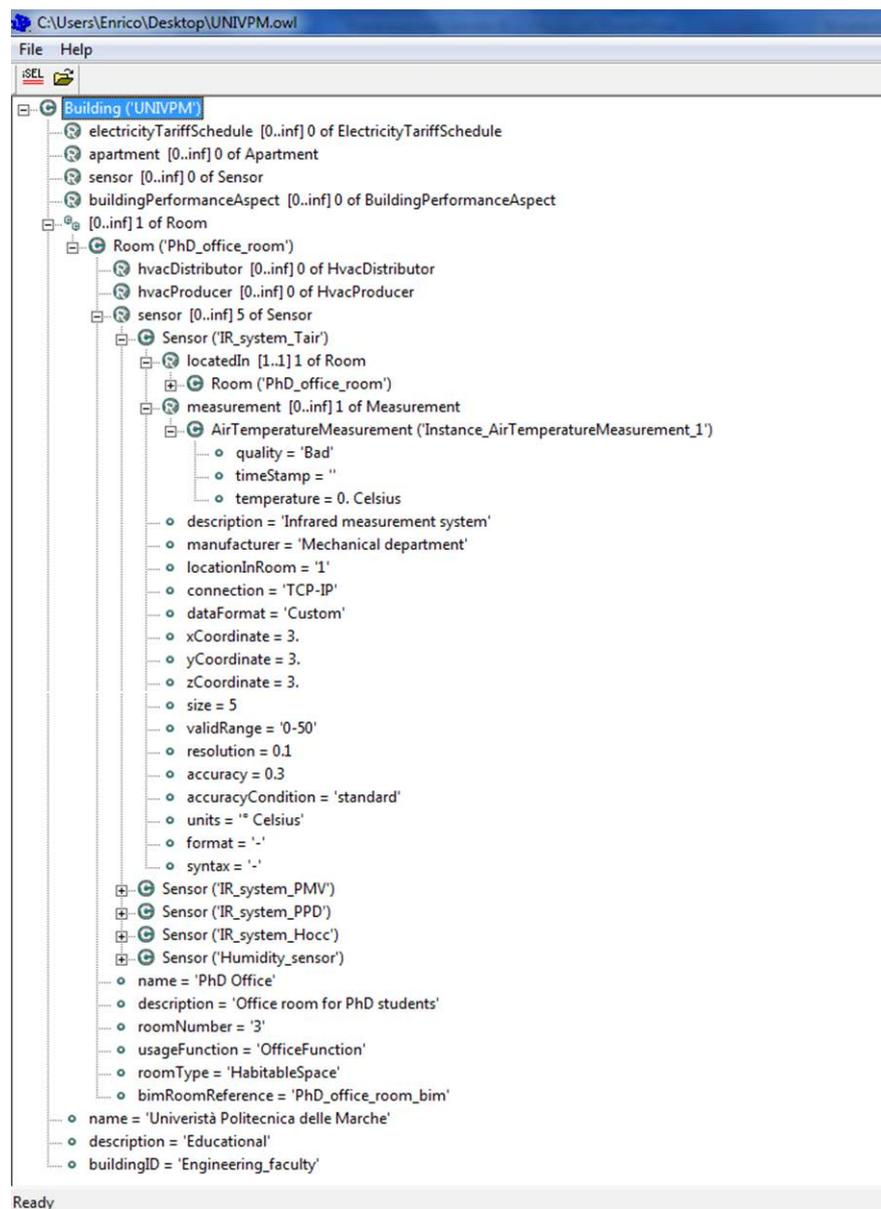
Figure 7: IR system parameters in implemented ontology instance
