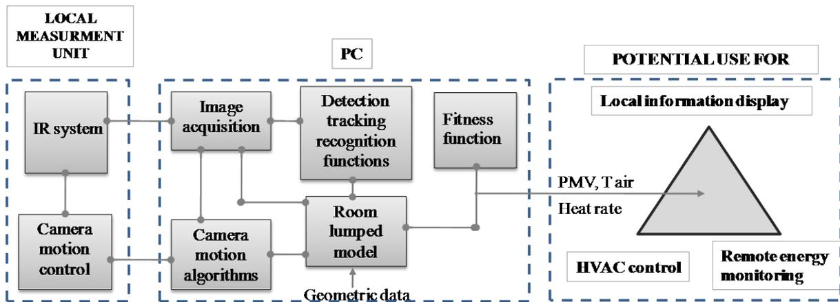
Figure 2: System components and functionalities of the IR-based system
