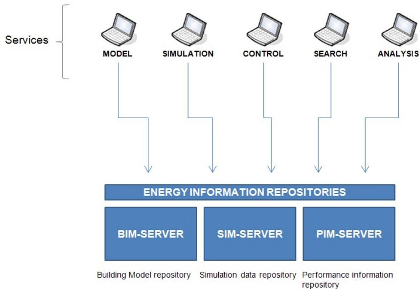
Figure 4: Energy Information Integration Platform (EIIP) concept.
